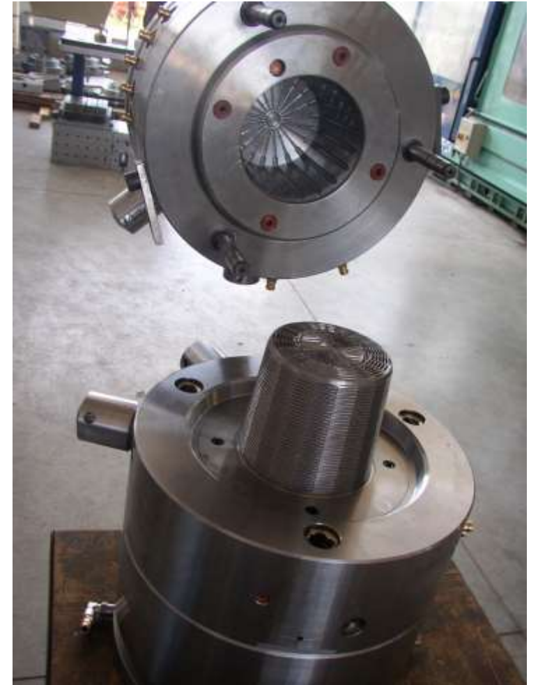
Mould for cheese container Mould dim.: Ø385x548 Mould weight: 497 Kg.
