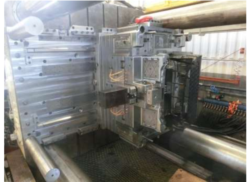
SKODA Flow Regulator with double fix side and translating moving side
