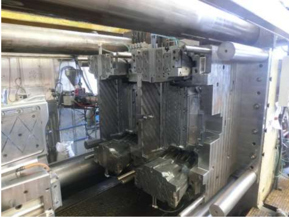
SKODA Flow Regulator with double fix side and translating moving side
